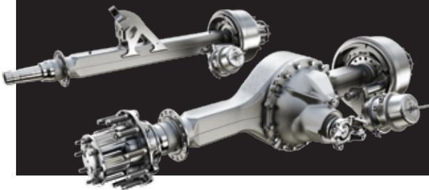
*A powertrain that pulls strong down low needs a fast axle, which is why we offer 6x2 single drive with tag axle and 6x4 tandem axles. These axles were **integrated** specifically with the downsped DD15 and DT12, to give you the performance, power and fuel economy you need.*
