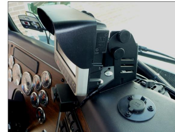
AWTI Camera Mounted using common mounting pattern
